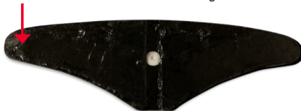
Electrode with Gel Missing
